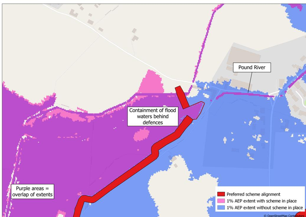
Example of containment - retaining water on the Pound River system
