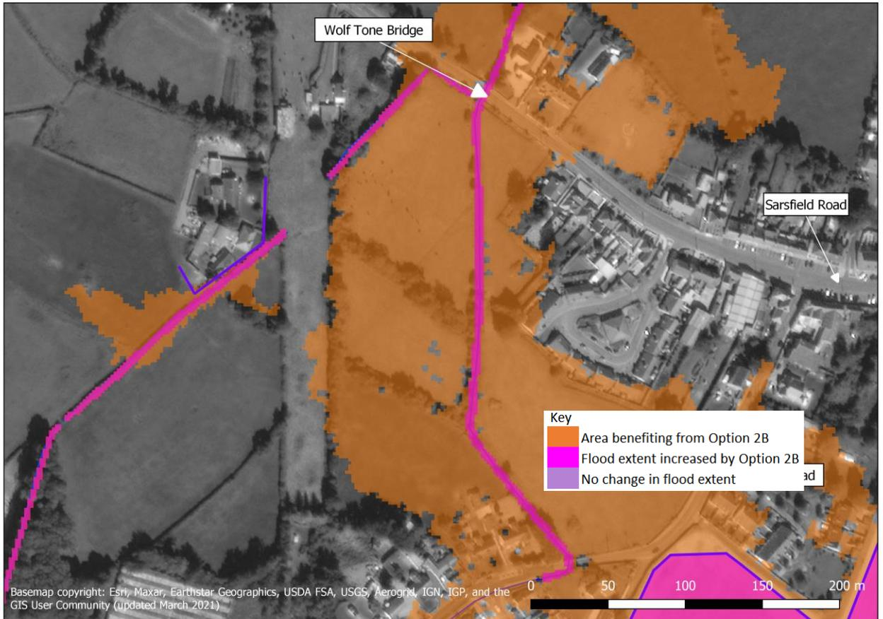
**Description:** In Option 2B, the combination of the main Owenass embankment and the Pound embankment and throttle means there is no flooding modelled in this area. Therefore there is no need for defences along Wolfe Tone bridge or around the property boundaries.
